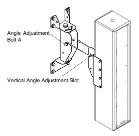
5. Lightly turn clockwise two axis bolts A to secure Speaker Brackets L and R. Set the speaker's vertical angle, and tighten the adjustment bolts A and axis bolts A.
