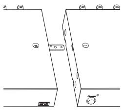
**Step 3.** Fix 2 units together using the remaining 2 joint bars and CSK screws (M3 x 6) on their bottom side.
