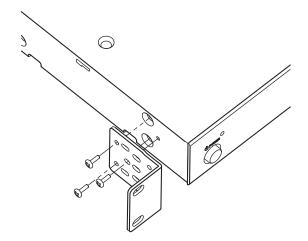
**Step 2.** Remove 3 case holding screws (M3 x 6) from the right hand side of the unit's case (viewed from front), and mount the long mounting bracket (having 2 antenna inputs) using the screws.
