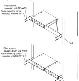
To mount two units in an equipment rack, use the optional MB-WT4 Rack Mount Kit.
