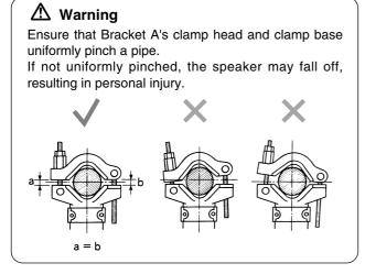
Pinch the pipe with Bracket A, and tighten both the lock nut and loose joint prevention nut.
