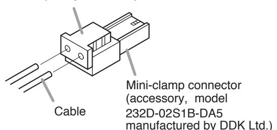
**Step 2.** With a pair of pliers, lightly pinch the mini-clamp cover and, after ensuring that the cable is securely inserted, firmly squeeze on the cover.
