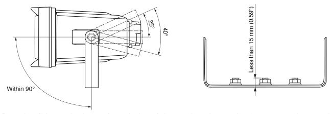
• Do not install the speaker face-up from a horizontal plane nor in such a way that the paper cone is exposed to direct sunlight.
