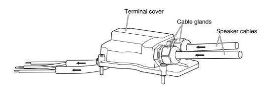
**Step 5.** Connect the speaker cables with the same polarity to each terminal according to the polarity indication at the screw terminal.
