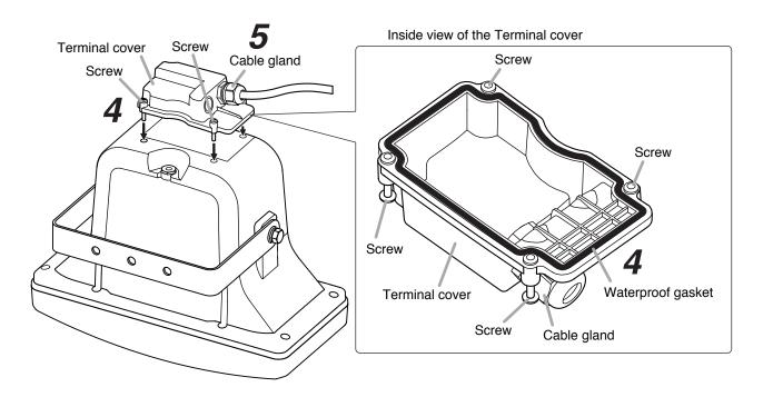
**Step 5.** Securely tighten the cable gland.
