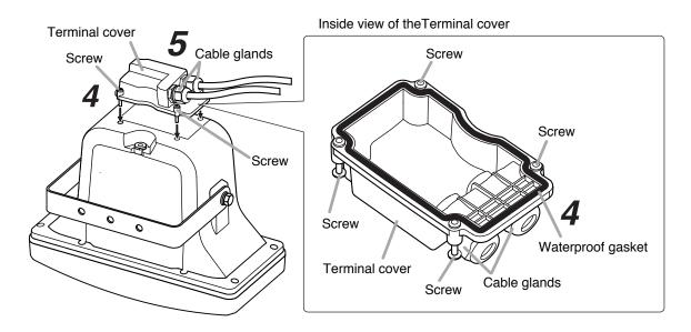
Step 7. Securely tighten the cable glands.
