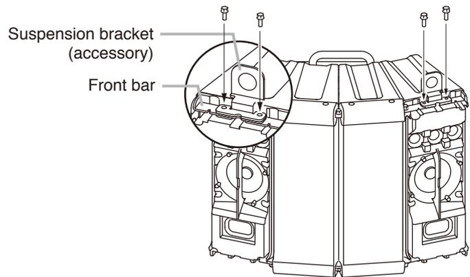
**Step 4.** For vertical suspension: Turn the speaker system upside down. Then, mount the suspension bracket in the same manner as described in **Steps 2 and 3**.
