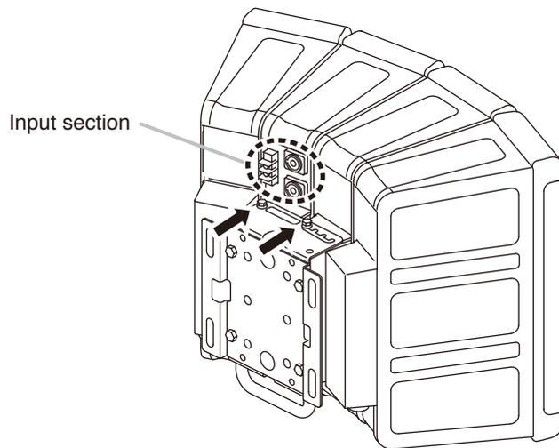
**Step 2.** Turn the speaker system upside down. Then, loosen the 4 bolts indicated by arrows.
