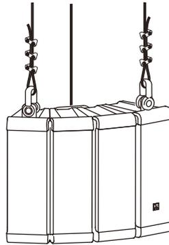
**Step 1.** For vertical suspension: Remove the speaker grill on the module to be suspended. (Below, upper)
