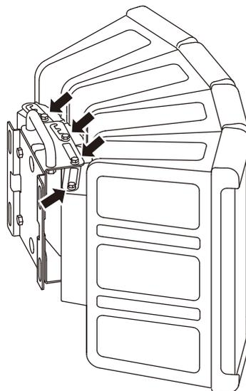
**Step 3.** Reposition the 4 bolts to the desired directivity angle, then retighten them securely.
