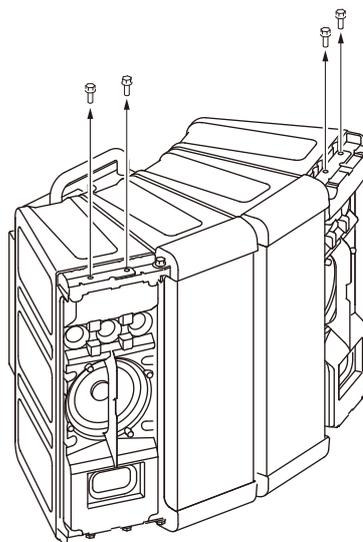
**Step 3.** Fix the suspension bracket and the front bar with the bolts removed in **Step 2**.
