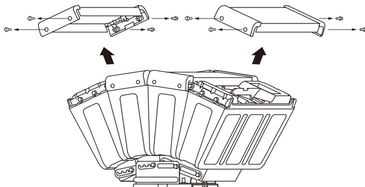
**Step 2.** For vertical suspension: Remove the 2 front bar fixing bolts. (Below, upper)
