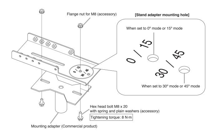
**Step 3.** Attach the mounting base to the angle bracket.
