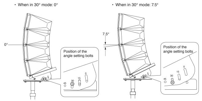
**7-1.** Loosen the angle bracket's fulcrum bolts and angle setting bolts.
