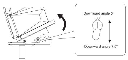
The figure shows the angle setting when in  $30^{\circ}$  mode. The downward angle can also be set similarly within the range of  $0^{\circ}$  to  $7.5^{\circ}$  when in  $0^{\circ}$  and  $15^{\circ}$  modes. However, the downward angle cannot be set when in  $45^{\circ}$  mode.
