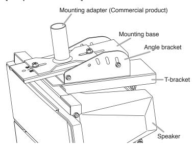
**Step 6.** Mount the speaker on the speaker stand (recommended product: K&M's 21300). Mount the speaker on the stand upside-down.
