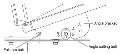
**7-2.** Lift the angle bracket, including the speaker with the fulcrum bolt as a fulcrum, so that the required downward angle can be obtained.
