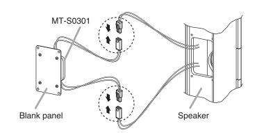
Step 5. Replace the blank panel with the matching transformer fixed in the speaker.
