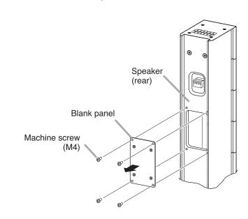
Step 2. Mount the matching transformer to the back side of the blank panel with the machine screws and nuts attached to the blank panel.
