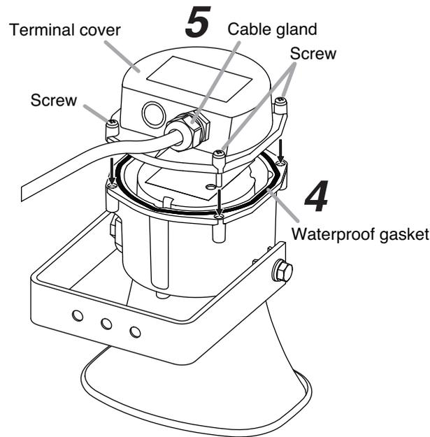
**Step 5.** Securely tighten the cable gland.
