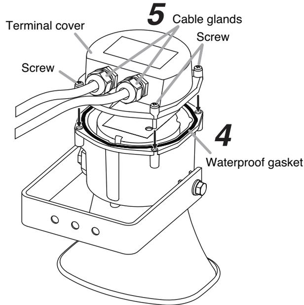
**Step 7.** Securely tighten the cable glands.
