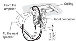
Step 6. Push the ceiling cover, slipped over the cord in Step 2, onto the ceiling surface, then tighten the cover-retaining nut using a 17 mm (0.67") hex wrench.
