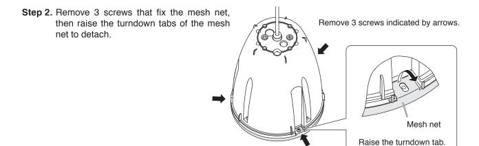
**Step 3.** Clean the speaker cover and mesh net. Wipe with a soft cloth damped in a detergent.
