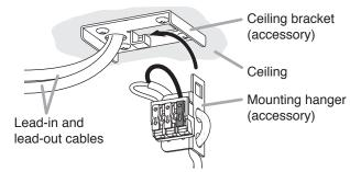
**Step 5.** Connect both the lead-in and lead-out cables to the input connector.
