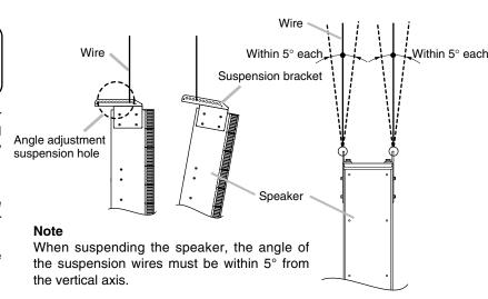
The mounting position for the suspension bracket can be moved up to 20 mm back and forth, permitting fine adjustment of the suspension angle.
