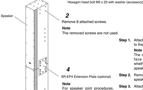
Remove 8 attached screws.
