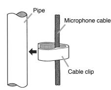
After putting a microphone cable in the supplied cable clip, attach the clip to the pipe.
