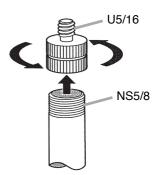
Removing a thread adaptor (U5/16) permits installation of a NS5/8 microphone holder.
