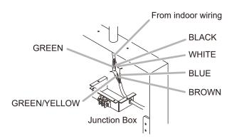
**Step 4.** Attach the junction box to the back box using the supplied screws as shown below. The BX-9F differs from the BX-9S in the way to attach the junction box to the back box.
