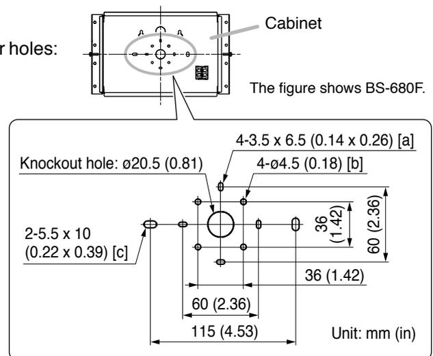
**2-3.** When mounting the cabinet into the wall:
