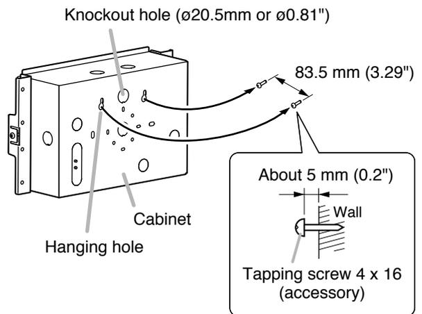
**2-2.** When installing the cabinet on the wall using other holes:
