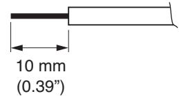
**4-3.** Connect speaker cables to the output terminals.
