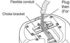
Plug the wired input connector into the speaker's socket, then pull the speaker cable from the choke bracket. (For wiring the input connector, refer to p. 10.)
