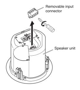
Step 3. Insert the stripped cable end into the terminal and tighten the terminal screw with a screwdriver.
