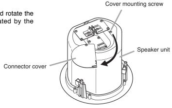
**Step 2.** Detach the removable input connector from the speaker's socket, and loosen the screw of the terminal to be used.
