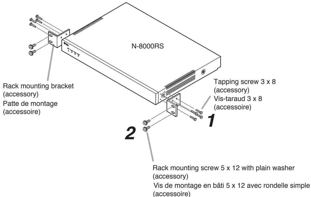
**Step 1.** Install the rack-mounting bracket to the N-8000RS.
