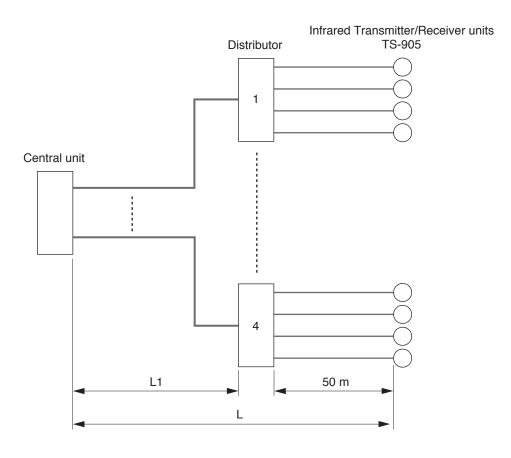
The equation and maximum cable length in this example are the same as those in Example 2 in the previous section on p. 61.
