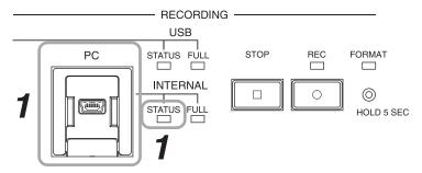
**Step 1.** Connect a PC to the PC Connection port.
