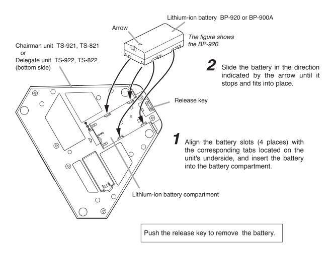
Note: A fully charged battery can be continuously used for about 10 hours.
