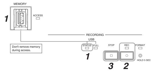
**Step 1.** Confirm that no USB memory device is inserted in the USB memory port and that the Internal emory status indicator is lit green.
