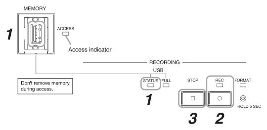
Step 1. Insert the USB memory device into the USB memory port.
