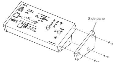
**Step 2.** Attach the MB-TS920 Rack mounting bracket to both sides of the Central unit. Use the screws removed in **Step 1.**
