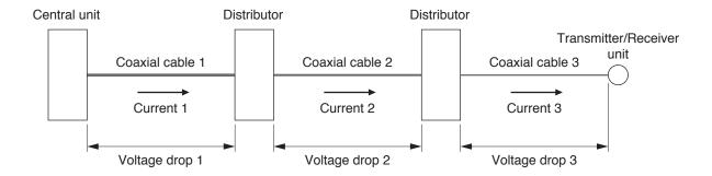
**Note:** For the coaxial cable required to carry a large current, use a cable of low loop resistance type.
