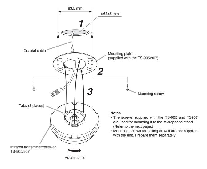
Step 1. Make a 68 mm diameter hole in the ceiling.
