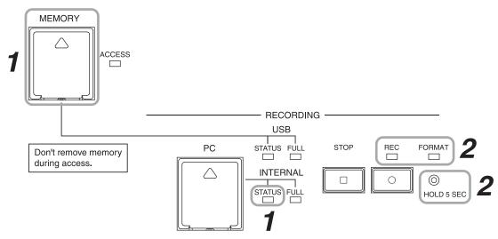
**Step 1.** Confirm that no USB memory device is inserted in the USB memory port, and that the Internal Memory status indicator is lit green.
