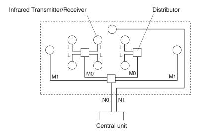
When two or more Infrared transmitter/receiver units receive infrared signals from the Infrared conference units, the signal reception level increases if input signals to each Transmitter/Receiver unit are in phase. If not in phase, the signal reception level may decrease.
