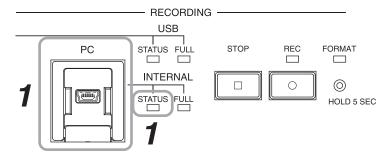
**Step 1.** Connect a PC to the PC Connection port.
