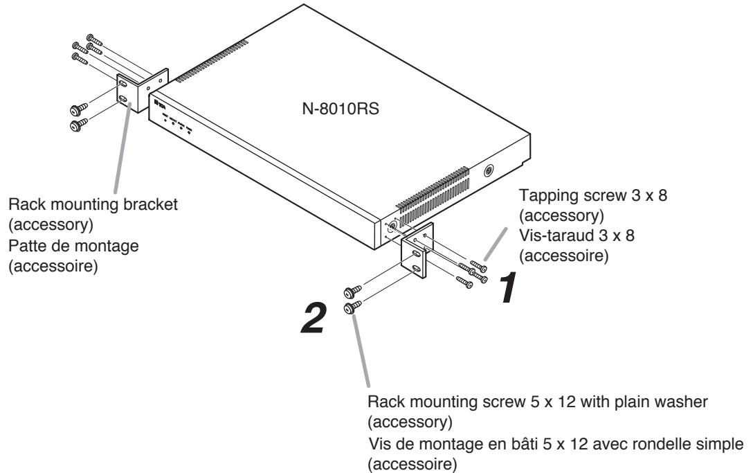
**Step 1.** Install the rack-mounting bracket to the N-8010RS.
