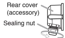
**Step 2.** Remove both the sealing clamp and the sealing bush from the recess in the cover.
