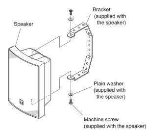
Step 2. Mount the speaker in the desired location using the mounting holes made in the bracket.
