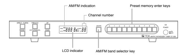
**Step 1.** Press the AM/FM Band selector key to select either AM or FM broadcast. The selected band is displayed on the screen.
