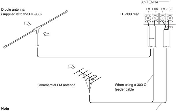
The antennas can receive radio signals at the highest level from the direction indicated by the arrows.
