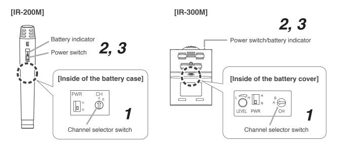
Step 1. Confirm that the infrared wireless microphone has been set to the same channel as that of the infrared wireless tuner. (Refer to p. 11 "CHANNEL SETTINGS.")
