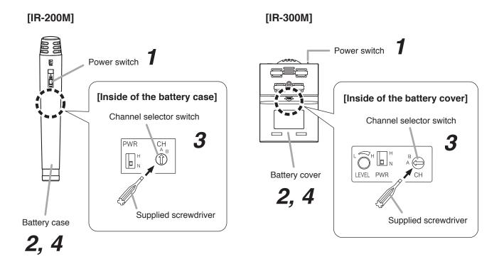
Step 1. Set the power switch to the OFF position.
