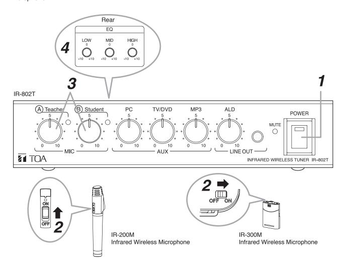
**Step 1.** Turn on the unit's power switch. The power indicator lights.
