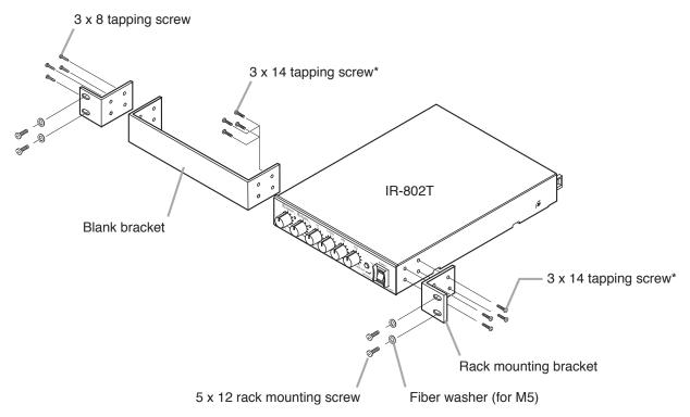
\* Secure the brackets with the screws supplied with the MB-15B-BK after removing the case holding screws, which are no longer used.
