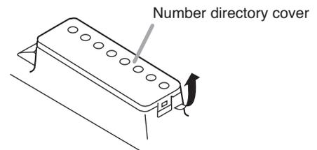
**Step 2.** Remove both the number directory cover and the directory. Remove the handset hook and reverse its orientation, then replace.
