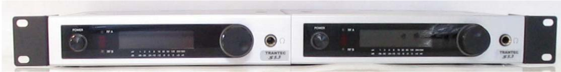
The rack mounting kit is supplied as standard with S5.5 systems, or is available as an accessory for S5.3 systems.
