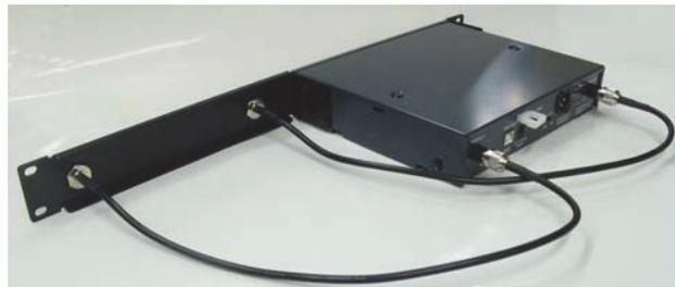
3. Fit the 2 supplied antenna extension cables into the front panel long bracket and tighten their BNC nuts. Screw the BNC plugs of each into the antenna sockets on the rear of the receiver. Should front mount antennae not be required, fit the 2 plastic blanking plugs supplied into the spare holes.
