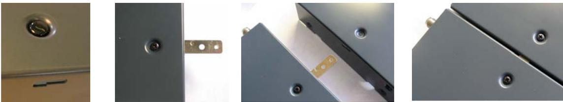
3. Fit 2 joining strips across the bottom of the receiver chassis using 4 M3x6 CSK screws (2 supplied per receiver).
