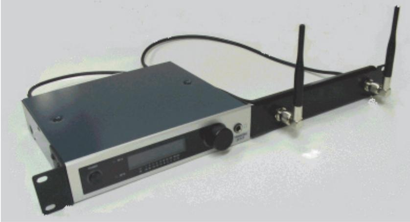
1. Unscrew 3 x lid retaining screws (M3x6) from the front left side of the chassis (viewed from the front) and fit the small angled rack bracket, using the supplied screws. There are 3 of these supplied with each receiver.
