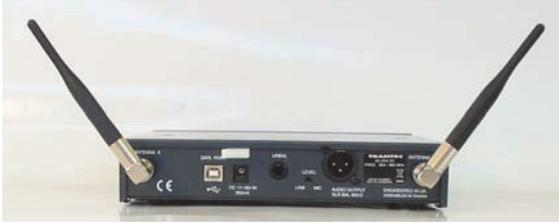
1. Attach the 2 supplied antennae to the rear panel BNC antenna connectors as shown left.
