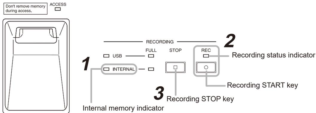
**Step 1.** Confirm that no USB memory device is inserted in the USB memory device port and that the Internal memory indicator is lit green.
