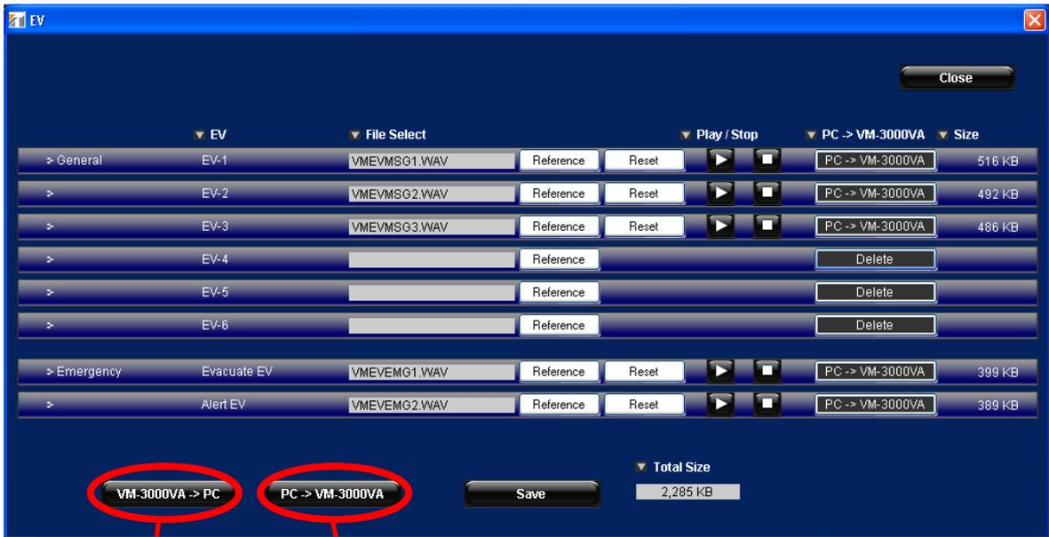
Press the [PC->VM-3000] button to transmit sound source data from the PC to the VM-3240VA/3360VA/3240E/3360E after reading the sound source data into the above screen.
