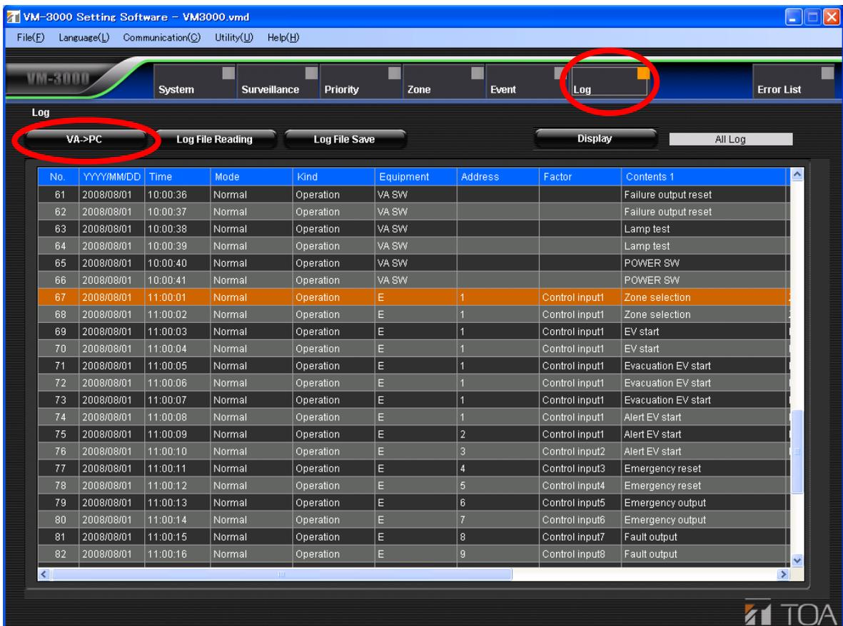
Pressing the [VA → PC] button starts the transmission of log data from the VM-3360VA or VM-3240VA to the PC.
