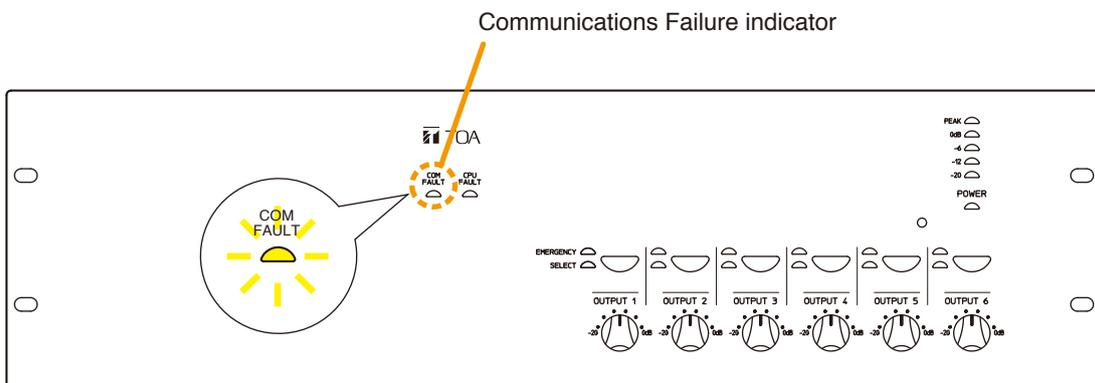
A failure has occurred in communications between the unit and the VM-3360VA or VM-3240VA. The previous status is automatically restored if communications return to normal.
