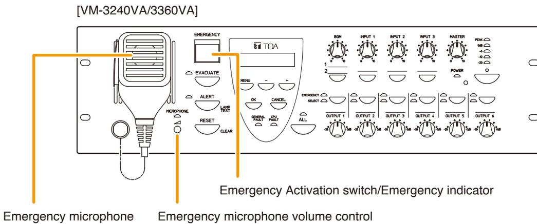
While the Emergency Activation switch on the front panel of the VM-3360VA or VM-3240VA and the Emergency Microphone's Talk key are simultaneously held down, the Emergency indicator (red) remains lit and the amplifier is placed in CPU OFF condition, allowing all-zone calls to be made from the Emergency Microphone. Adjust the sound volume with the Emergency Microphone's volume control.
