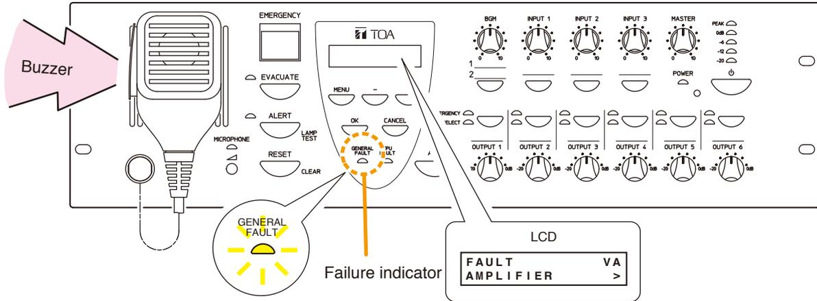
In this event, a failure of the contents shown on the LCD screen has occurred within the system. Pressing the amplifier's [OK] key to acknowledge the failure or acknowledging the failure by way of the Fireman's Microphone stops the buzzer and switches the yellow failure indicator from flashing to steady-on mode. (Refer to "Failure acknowledgment" on p. 57).
