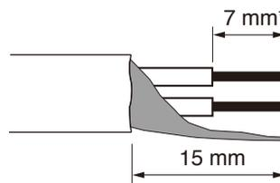
\* Expose 8 mm or more when using the above ferrule terminal, and cut off an extra conductor protruding from the sleeve.
