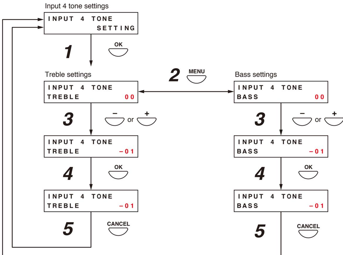
**Step 1.** Press the OK key on the Input 4 Tone Settings screen. The Treble Settings screen is displayed.
