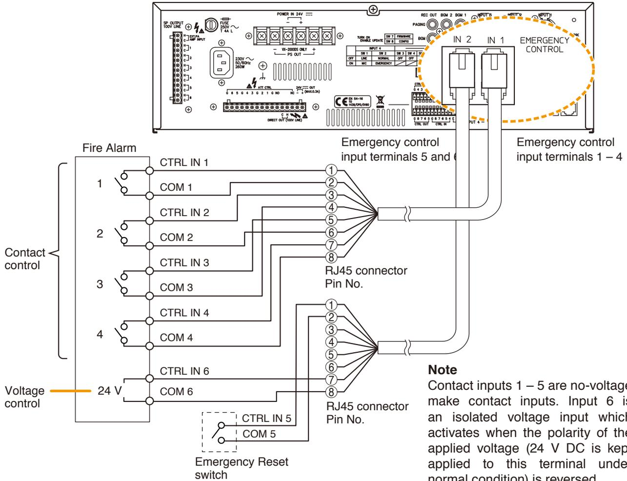
[Terminal assignment to the emergency control inputs]
