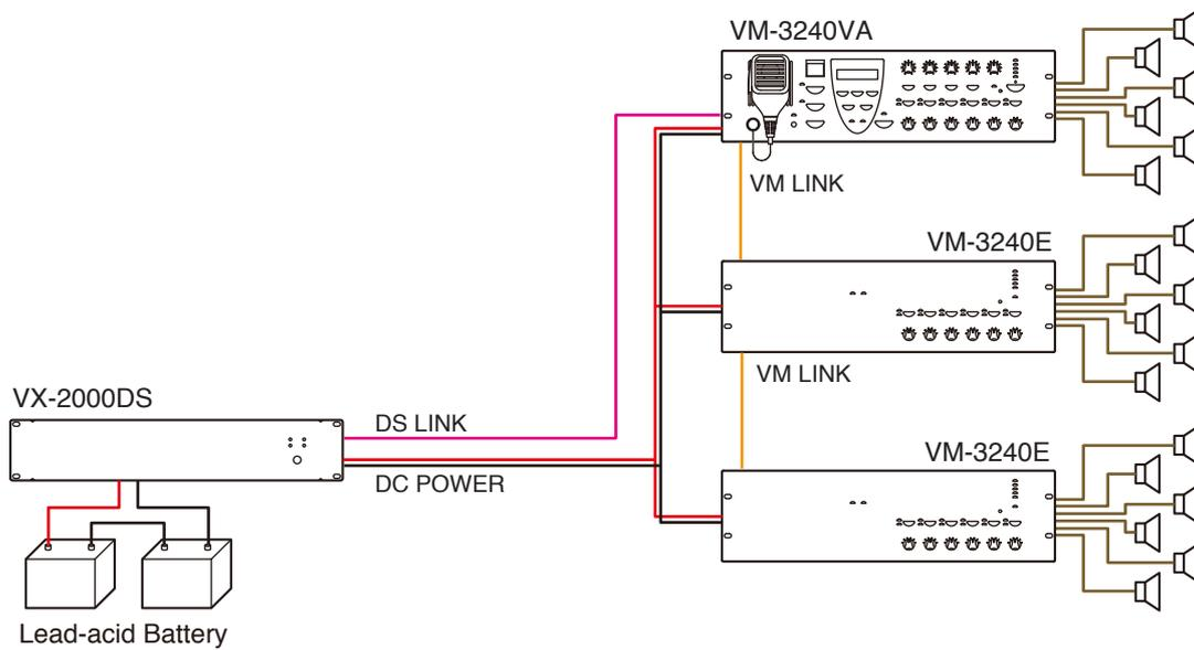
**System including one VP amplifier connected as a standby amplifier**
