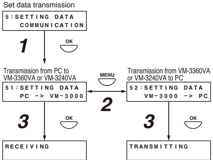
**Step 4.** Activate the setting software to transmit set data from the VM-3360VA or VM-3240VA to the PC or from the PC to the VM-3360VA or VM-3240VA. Click "Communication" on the menu bar and select "Setting Data: VA->PC" or "Setting Data: PC->VA" on the pull-down menu.
