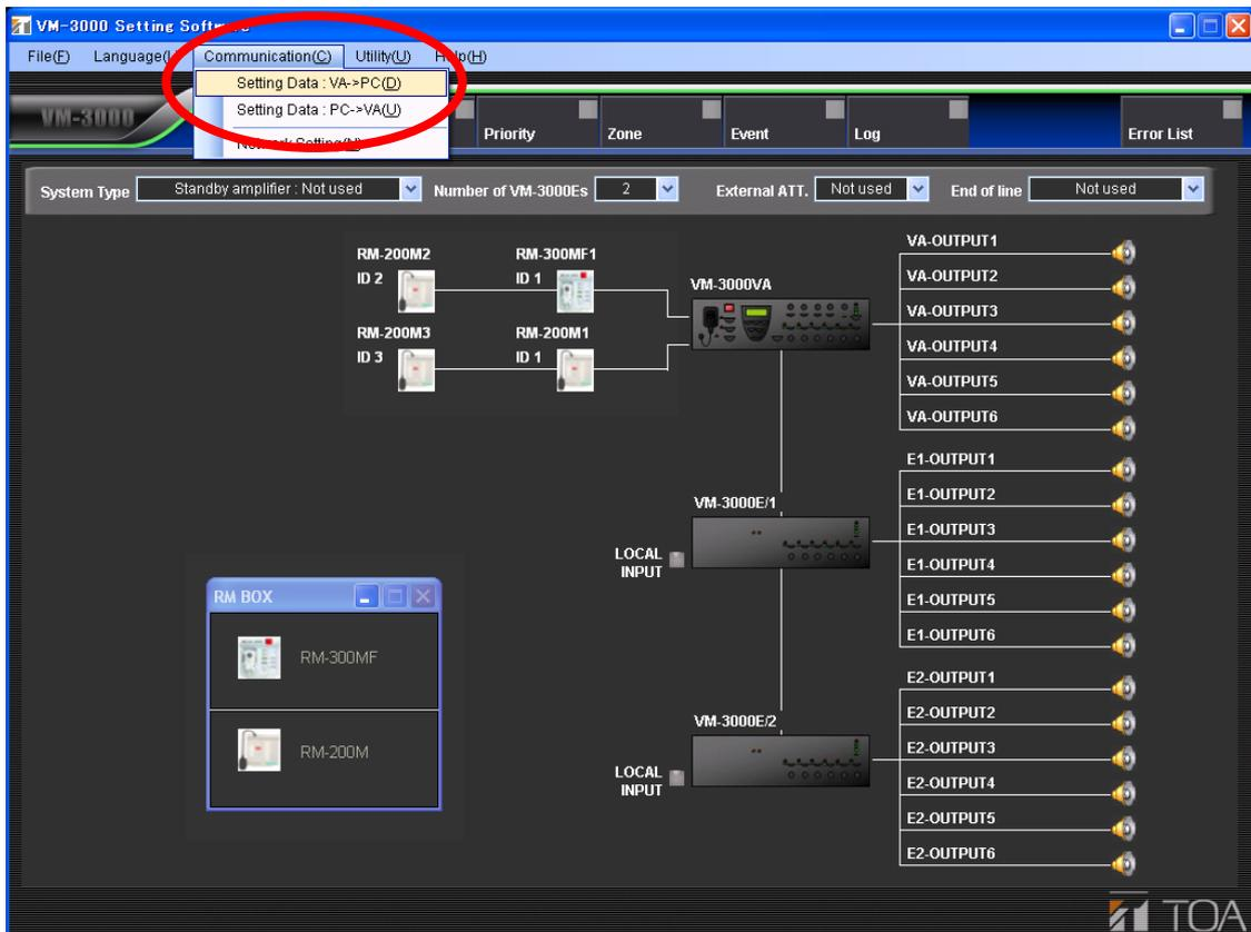
Selecting "Setting Data: VA->PC" allows PC-set data written to the VM-3360VA or VM-3240VA to be read into the software.
