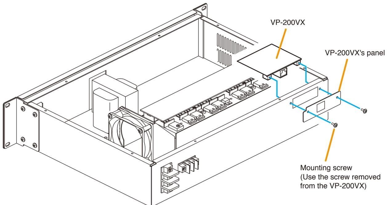
**Step 4.** Plug the VP-200VX's connector into the CN106 connector on the circuit board inside the amplifier.
