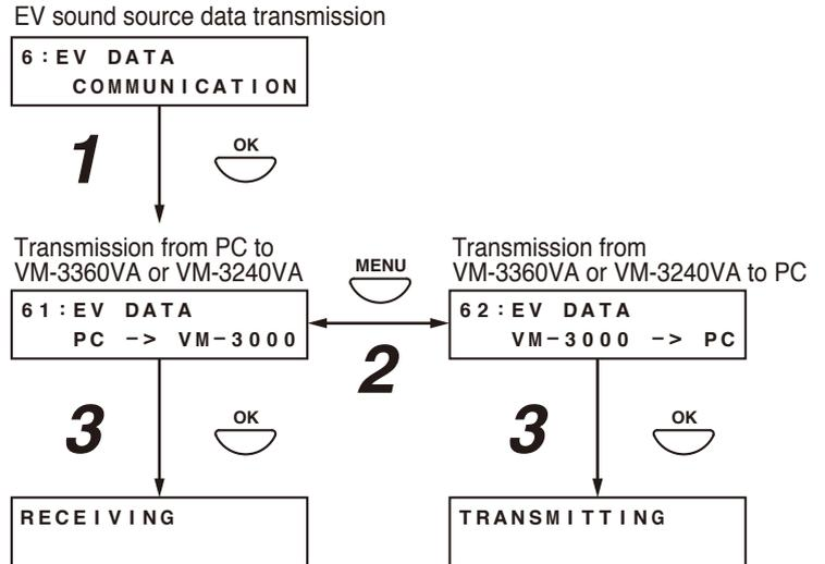
**Step 4.** Activate the setting software to transmit the EV sound source data from the VM-3240VA/3360VA/3240E/3360E to the PC or from the PC to the VM-3240VA/3360VA/3240E/3360E, then click "Utility->EV" on the menu bar.
