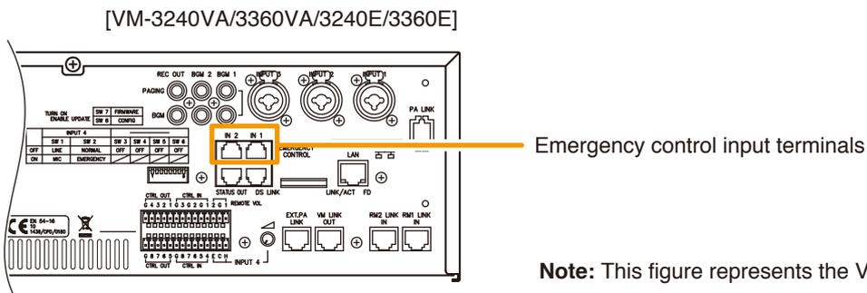
**Step 2.** The Alert or Evacuation announcement is broadcast over the zone(s) assigned to the Emergency Control Input terminals. The Emergency indicator flashes red, the buzzer sounds and the Alert or Evacuation Announcement indicator lights red. At the same time, the Output indicator corresponding to the set broadcast zone(s) lights.
