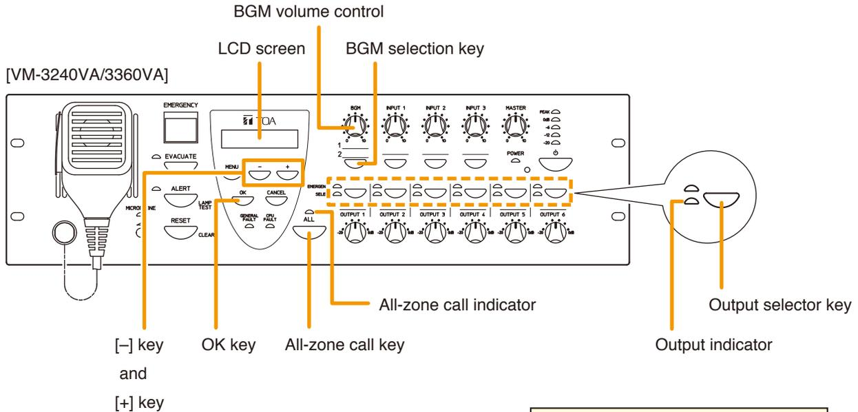
**Step 1.** Press the BGM selection key. The "Select BGM" screen will be displayed on the LCD.
