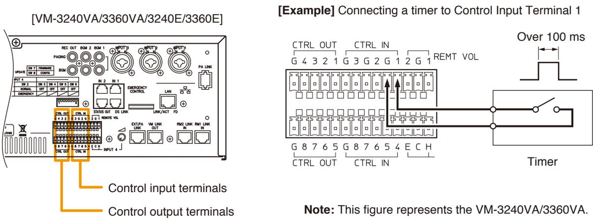
**Step 2.** When the timer's preset time is reached, the Contact Input receives a contact output signal (make contact) from the timer. The all-zone call indicator or output indicator corresponding to the set zone lights green and the automatic general announcement is broadcast over that zone.
