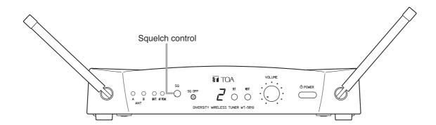
The WT-5810 tuner has the squelch function that virtually eliminates ambient noise and unwanted audio signals from other wireless microphone systems by silencing the output when the signal received is lower than a certain level of signal strength.
