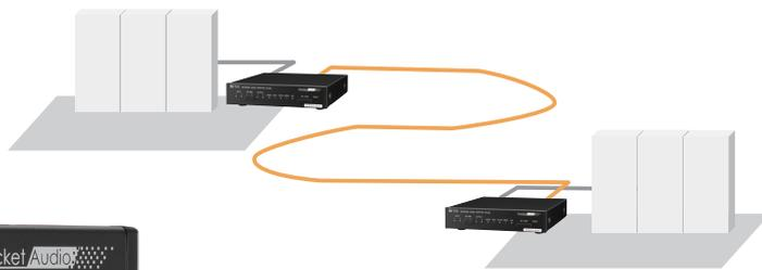
NX-300 Network Audio Adapter can convert audio signals to high quality digital signals. Regardless of the geographical distance, the digital signals can be transmitted simultaneously over the IP networks, such as LAN or Internet. The contact closure can operate the distant devices via the network.
