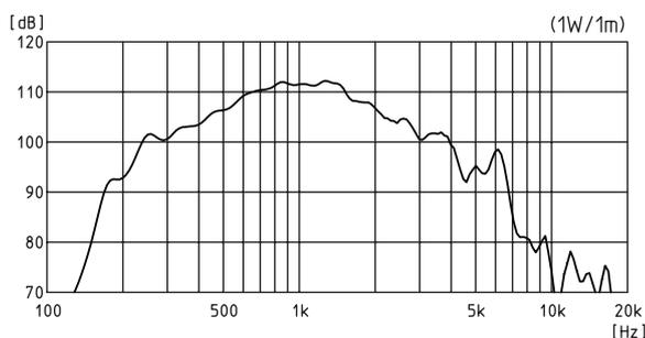
Improving these high and low range frequency characteristics is one of the issues key to improving horn speaker sound quality. Particularly, we now understand that improving the high range contributes greatly to improving the articulation of outdoor broadcasts. Attenuation in the air is more conspicuous for the high frequency ranges.
