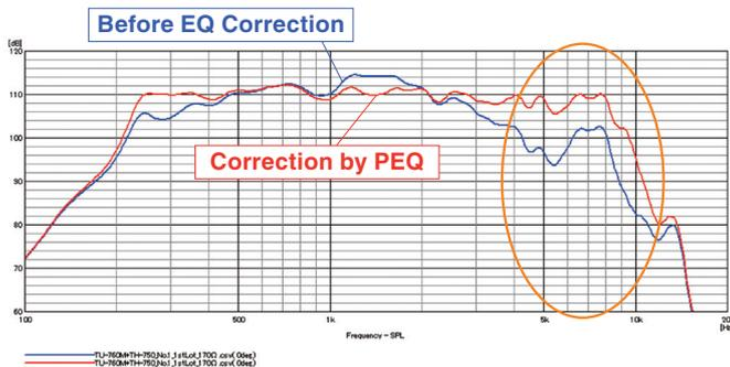
Because the TU-660 allows high range reproduction, it is possible to use EQ to raise SPL around 5-8kHz. Further, by suppressing SPL around 1-2kHz, flat characteristics can be achieved even in a horn speaker.
