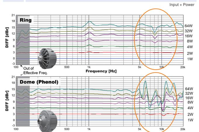
The graphs above compare the linearity of frequency characteristics against input power levels for the ring-type TU-660 construction (above) and dome-type construction of other driver units (below).
