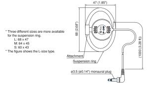
YP-E401 Ear-suspension Earphone is 3.5 mm in plug diameter, and 16  $\Omega$  in impedance.
