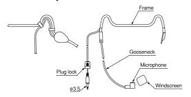
WH-4000H is headset microphone of a cardioid pick-up pattern, featuring a lightweight design.
