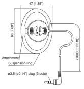
YP-E5000 is Assist Earphone is 3.5 mm in plug diameter, and 16  $\Omega$  in impedance.
