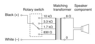
**Note:** The rotary switch is factory-preset to  $1.7 \text{ k}\Omega$ .
