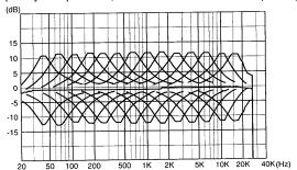
• Frequency Response (ex. All slider is set at a max. or min. position)
