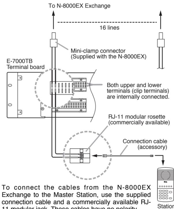
To connect the cables from the N-8000EX Exchange to the Master Station, use the supplied connection cable and a commercially available RJ-11 modular jack. These cables have no polarity.
