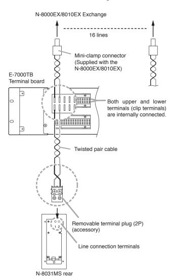
To connect the cables from the N-8000EX/8010EX Exchange to the N-8031MS, use the removable terminal plug (2P) supplied with the N-8031MS. The cables have no polarity.
