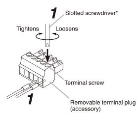
\* Recommended type of screwdriver with the following blade width: For 5P terminal plug: About 2.5mm (0.1") wide blade For 3P terminal plug: About 3.5mm (0.14") wide blade
