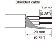
\* Expose 8 mm (0.31") or more when using the above ferrule terminal, and cut off an extra conductor protruding from the sleeve.
