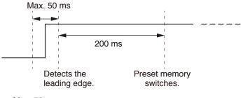
(B) Opening the contact terminal after the Preset memory has been switched.
