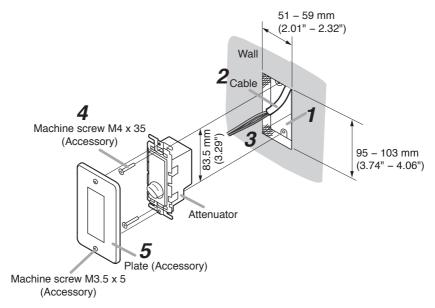
Note: When using the supplied screws to install the unit to the electrical box, the distance between the wall surface and the electrical box's surface should be less than 27 mm (1.06") as shown below.
