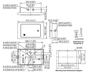
\*Since no mounting screws are supplied with the speaker, separately prepare them appropriate for the construction of wall and its thickness
