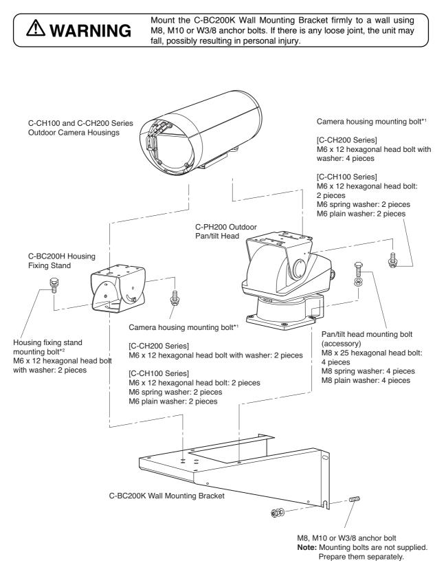
\*1 Supplied with the C-CH100 or C-CH200 Series Outdoor Camera Housings.
