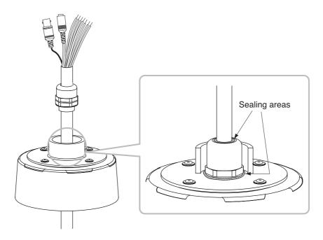
4. Replace the connectors removed in Step 1 on the end of the composite cable.
