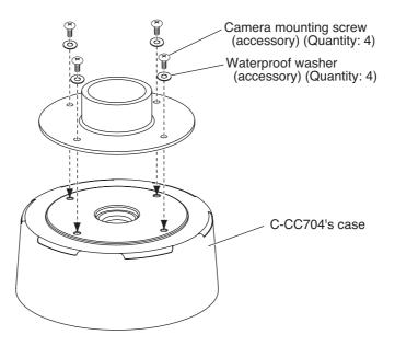
3. Secure the cable bushing into the upper side of the pendant adapter while running the free end of composite cable through the C-CC704's case from the upper pendant adapter.
