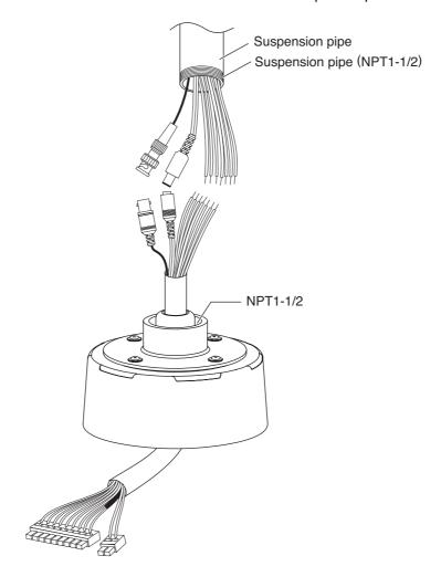
6. Waterproof the suspension pipe threads after wrapping the sealing tape (supplied with the C-CC704) around them. Then, screw the pendant adapter assembled with C-CC704's case into the pipe.
