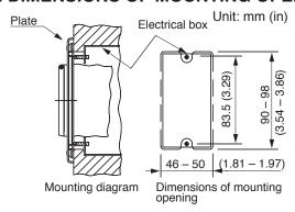
To fit the electrical box in the wall or ceiling, make opening according to the mounting dimensions shown at left.
