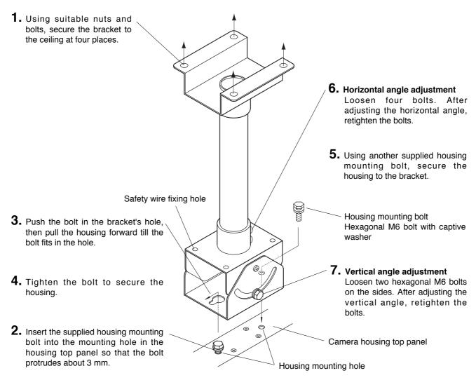
**Note:** The vertical angle adjustment bolts are loosely set when the unit is shipped from the factory. Be sure they are securely tightened after mounting the housing.
