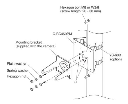
\*1 Use these holes to direct the camera in the panning direction.
