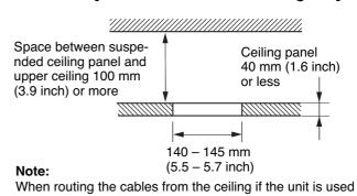
When routing the cables from the ceiling if the unit is used in conjunction with the N-CC2564, the ceiling panel must be 9 - 40 mm (0.4 - 1.6 inch) in thickness.
