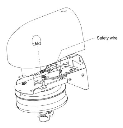
7. Attach both the inner cover and dome cover to the camera after camera adjustment completion. For details, refer to the instruction manual enclosed with the camera.
