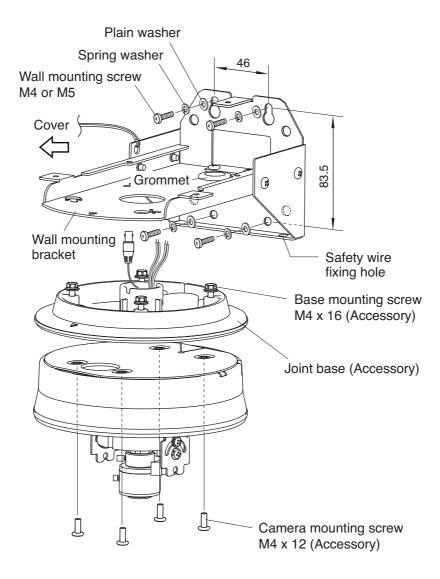
3. Fix the supplied M4 x 16 base mounting screws loosely to the joint base, then install the camera unit to the joint base using the supplied M4 x 12 camera mounting screws.
