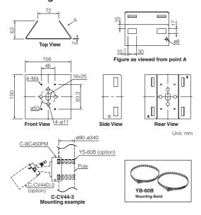
Designed to mount the C-CV44-3 on a pole in conjunction with the optional YS-60B.
