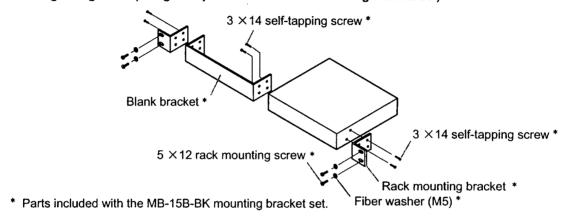
• Rack-mounting two units (using the optional MB-15B-J mounting bracket set)
