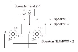
Two speaker systems can be operated in parallel by connecting them in a cascade configuration as shown at right.
